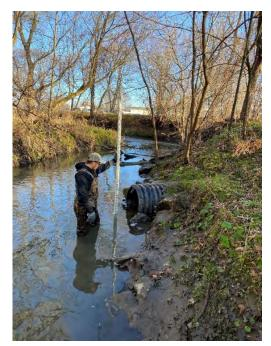
Figure 9.0: Sta. 12+00-12+50 Severe. Outfall is eroding, banks bare and channel is U-shaped.
