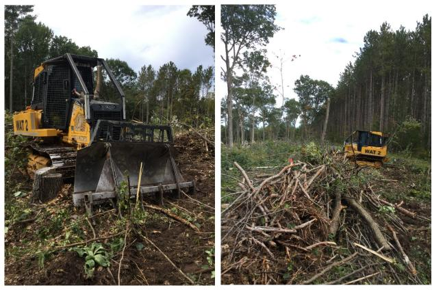
Figure 11. A WI DNR John Deere 450 LGP with a root rake attachment
