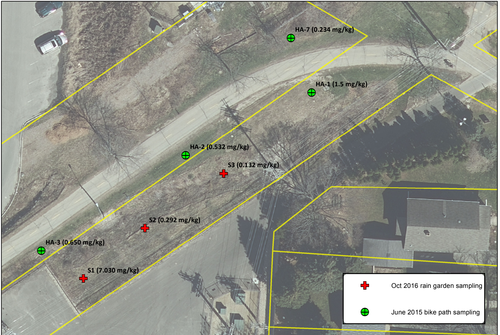
FIGURE 1 - PCB Sampling of Rain Garden Collected by City of Madison Engineering on October 19, 2016. Industrial Direct Contact Residual Contaminant Level is 0.744 mg/kg.
