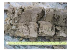
51.4 to 54.0' Clay, some silt, medium to high plasticity; trace small to large pebbles, subround to subangular up to 2" diameter; moist; stiff; dark grayish brown (10YR 4/2) NOTE: Lacustrine; laminated 0.01 to 0.02 feet thick, laminations brownish yellow (10 YR 4/3).
