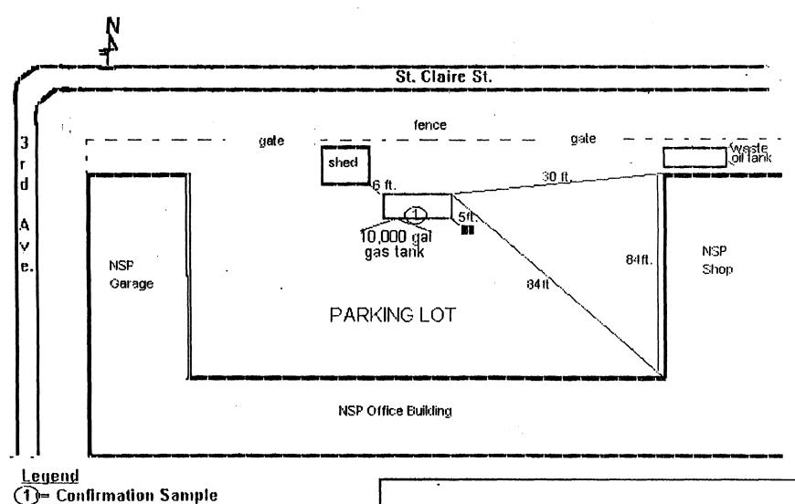
Tank dimensions: 30' L x 8' W Lab sample taken at 6.5 ft. FROM SOUTH SIDE WALL OF EXCAVATION
