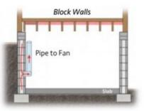
Informative advisory—If the top or wall surfaces of the void network cannot be closed to resist air entry into the voids, *depressurization* of the block wall(s) may not be possible. Where openings are not accessible, closure of voids in a course of blocks below the inaccessible openings at a location above outside grade should be considered to isolate a smaller void network for *depressurization*.
